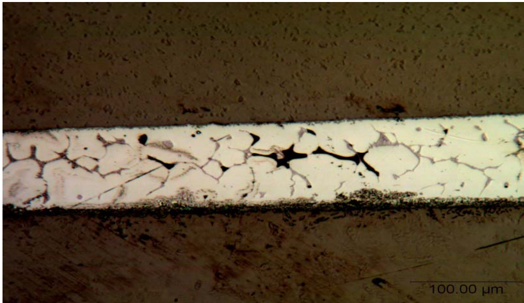
Fig. 3 CP Titanium plates (1 mm thick) torched brazed in air with TiBrazeAl-655 (Al-6.3Cu-0.3Mn-0.2Si-0.2Ti) filler metal using flux TBF-42. Gray and black phase in the joint is the Al-Cu eutectic [42]
