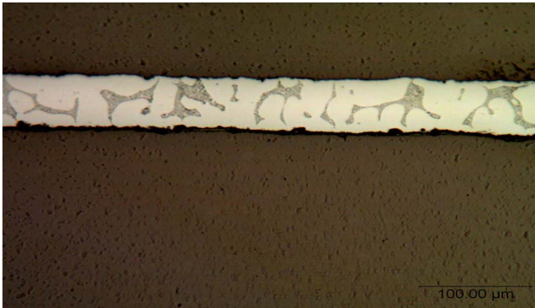
Fig. 4 CP Titanium plates (1 mm thick) torch brazed in air with TiBrazeAl-642 (Al-5.3Si-0.8Fe-0.3Cu-0.2Ti) using flux TBF-60 [42]
